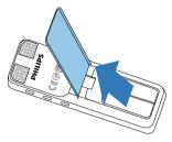
Insert the batteries or rechargeable batteries as shown into the device. Make sure the polarity is correct.
