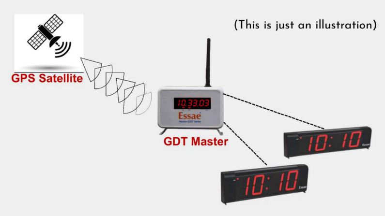
Wireless Transmission ......Satellite to Master [ Gps receiver and transmitter ] to Clocks
