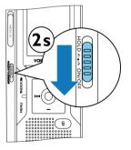
7 To power off, pull down the power switch on the side of the device again and hold for about two seconds.
